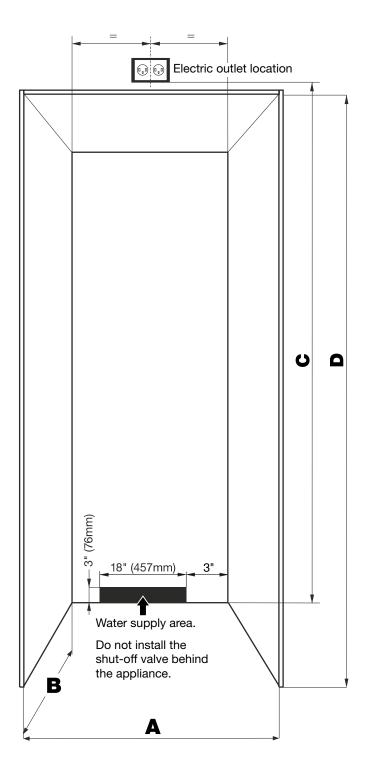
The appliance can be integrated into the kitchen units. To adapt the appliance to the height of the row of kitchen units, a suitable top cupboard can be fitted above the appliance.
